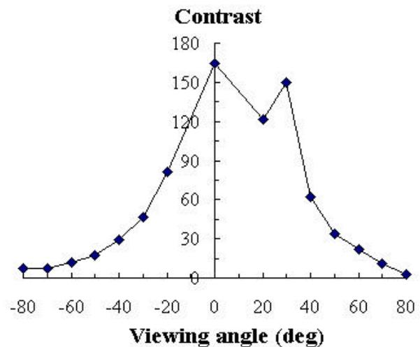
Fig. 5 Relationship between contrast and viewing angle in vertical direction.
