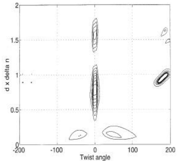
Fig. 2 Parameter space showing contours of iso-contrast ratio. ( $\alpha = 0^\circ$  with cross polarizers)
