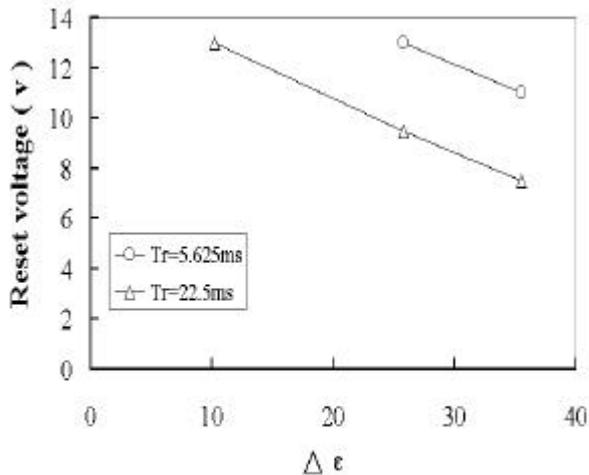
Fig. 6 Relationship between the reset voltage and  $\Delta \epsilon$  in difference reset time
