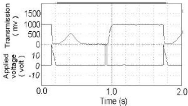
Fig.3 Time-dependent transmission and driving pulse curve of BTN cell with  $d\Delta n=0.78$ .
