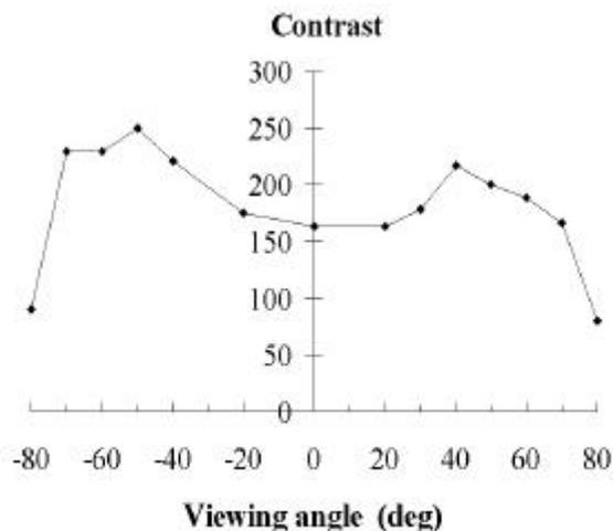
Fig. 4 Relationship between contrast and viewing angle in horizontal direction
