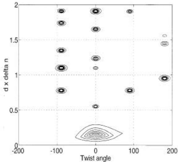
Fig. 1 Parameter space showing contours of iso-contrast ratio. ( $\alpha = 45^\circ$  with cross polarizers)
