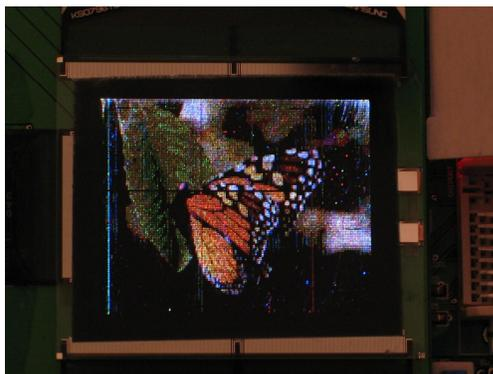
Figure 9. Photograph of an image displayed on a 2.1-inch MILC poly-Si TFT color AMOLED.
