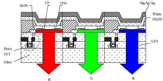
**Figure 6. Cross section schematic diagram to achieve color display by color filters and white OLED.**
