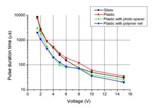
Figure 7: Relation between pulse duration and amplitude required to achieve bistable switching.
