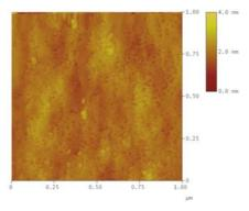
**Figure 3:** AFM picture of uncoated ITO covered PES substrate. The image size is  $1 \times 1 \mu m^2$  and the height scale is 4 nm.
