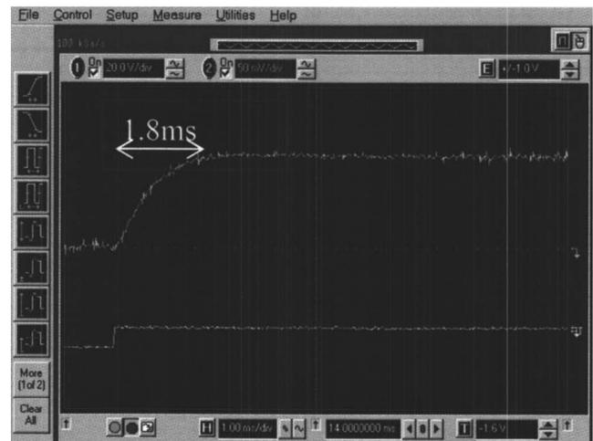
FIG. 4. Oscilloscope trace of switching of the NBB cell.
