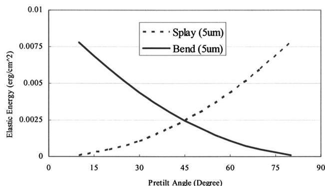
FIG. 1. Elastic deformation energies of the bend and splay cells as a function of the pretilt angle.
