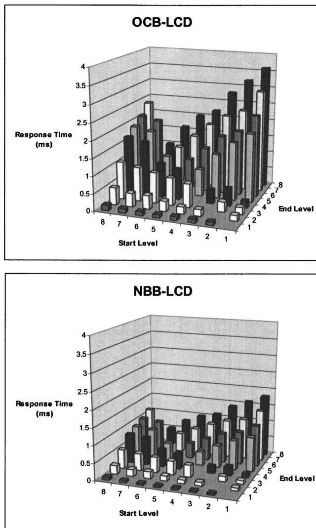
FIG. 5. Total switching times of the NBB cell and the OCB cell.
