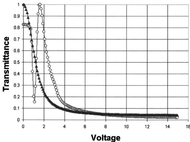
FIG. 2. TVCs of the NBB cell (triangles) and the OCB cell (circles). Both cells have the same thickness of 5 μm.
