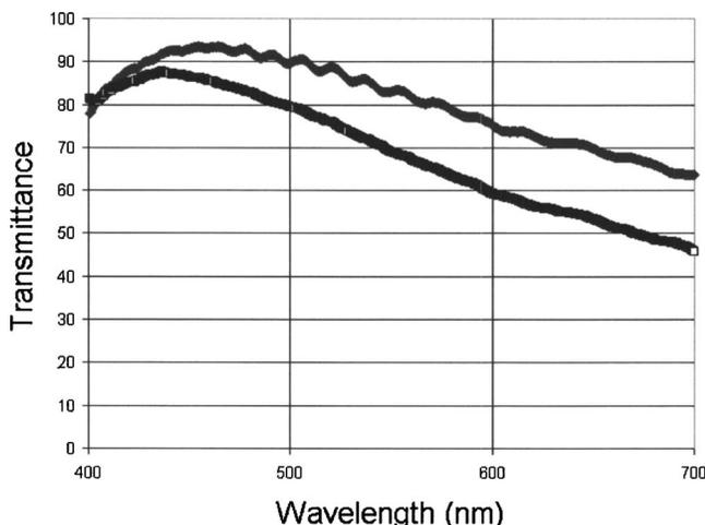
FIG. 3. Measured transmission spectra of the NBB cell and the OCB cell.
