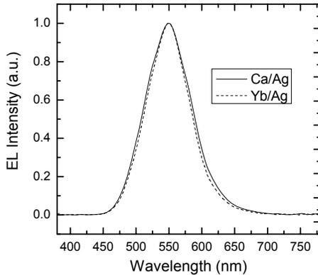
FIG. 3. Normal emission spectra of the TOLEDs with Ca/Ag cathode (solid line) and with Yb/Ag cathode (dashed line).
