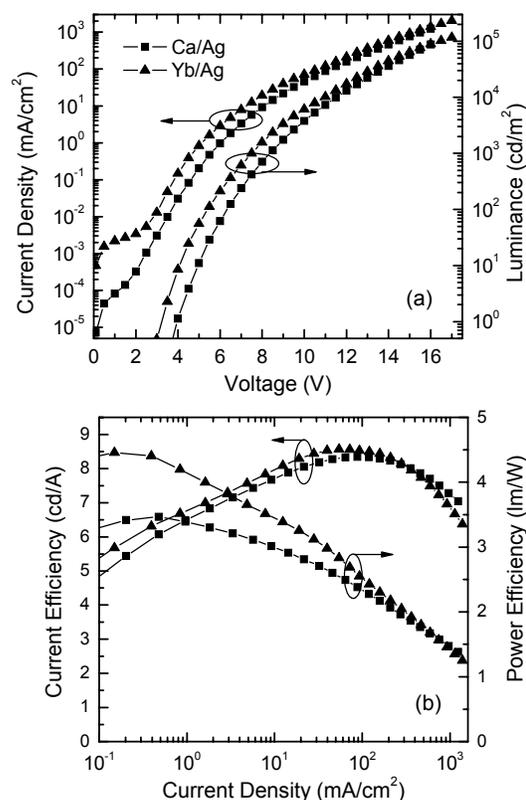
**FIG. 2.** (a) J-V-L and (b) efficiency characteristics of the TOLEDs with Ca/Ag cathode and with Yb/Ag cathode.
