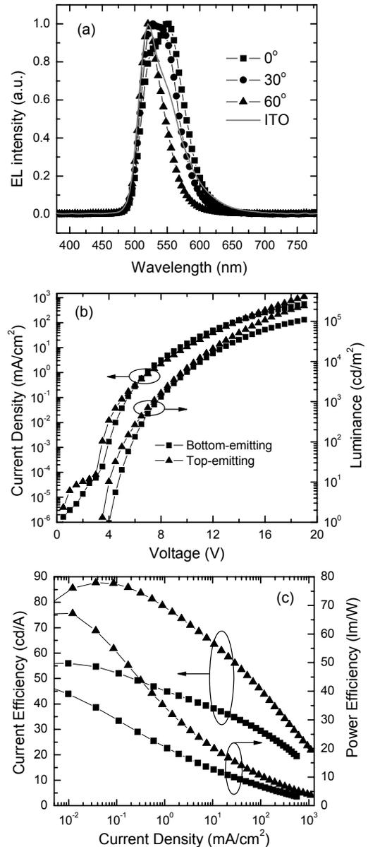
FIG. 4. (a) EL spectra of Yb/Ag based top-emitting device at different viewing angles in comparison with that from bottom-emitting device. (b) J-V-L characteristics of the top- and bottom-emitting devices. (c) Current and power efficiency comparison.
