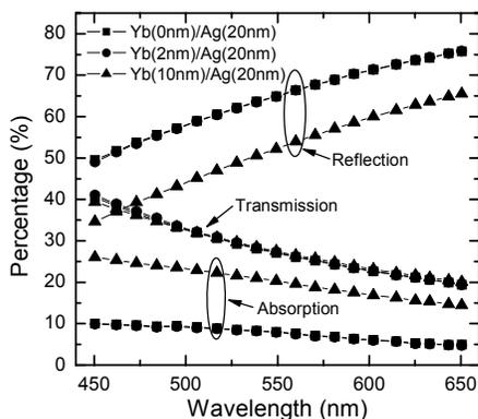
**FIG. 1.** Optical transmission, reflection, absorption of Yb(*x* nm)/ Ag (20nm) films.
