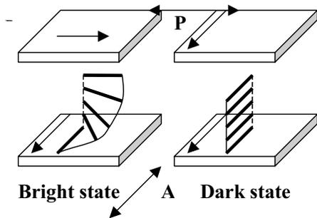
Fig.3 Principle of optically rewritable LC device
