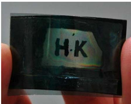
Fig.7 Demonstration of bending flexible optical rewritable reflective LCD
