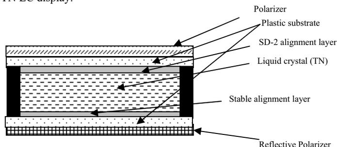
Figure 2. Cross section of flexible optically rewritable LC display
