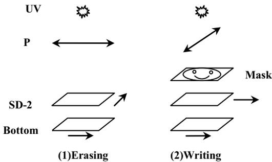
Fig.4 Principle of writing images in two processes
